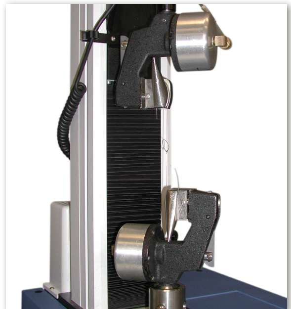
Figure 2: Suture material with a knot tied at the center of the specimen and loaded into the pneumatic cord and yarn grips for a knot-pull test.
