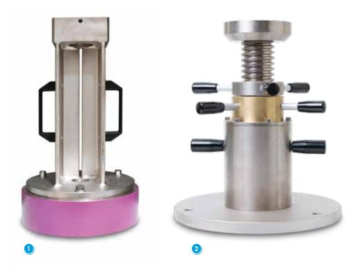
Test fixtures, a key component of the CEAST 9300 Series Drop Towers, are designed to test to a wide range of standards, components, and products. The fixture set includes a stand, where the specimen rests, and clamping mechanisms that push the specimen against the stand and hold it securely in place during an impact test.
