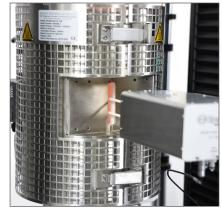
3119-160 Furnace combined with Instron's 3119-960 3 zone temperature controller ensures fast heat up times, accurate temperature control and full integration with Bluehill Universal Software.
