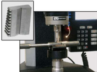
Soft materials, such as brass and magnesium, may require serrated jaw faces with as few as 4 teeth per inch. Gripping of medium hardness materials, such as sheet steel, is often done with serrated jaw faces having 16 to 25 teeth per inch. Harder steels may require smooth jaw faces coated with carbide particles called surfalloy. Match your jaw face selection to the hardness of the test specimen using the Rc 15 point rule to reduce slippage problems and extend your jaw face service life.
