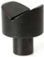
ASTM E18 is a good reference for anvil selection. The anvil must position the test specimen perpendicular to the indenter. A "V" style anvil is ideal for supporting cylindrical parts. A [cylindron anvil](#) is suitable for larger diameter parts. Elongated parts that extend beyond the frame should be supported with a Vari-rest type fixture to prevent part tilt or movement. Specialized anvils can accommodate varying geometries and radiuses.
