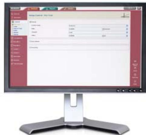
Better yet, we often recommend using a pre-load before the test starts if you know there will be some slack in your test setup or if your specimens exhibit some toe region in the data. You can set up Bluehill Software in the Control section of the Method tab to automatically apply a pre-load before data collection begins. This eliminates or minimizes the toe region and ensures
