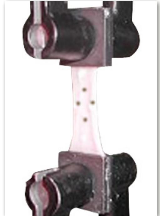
AVE marking using graphite-cyanoacrylate dots
