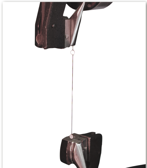
Figure 2: Close-up of the Nitinol wire specimen with white marks for tracking tensile strain.
