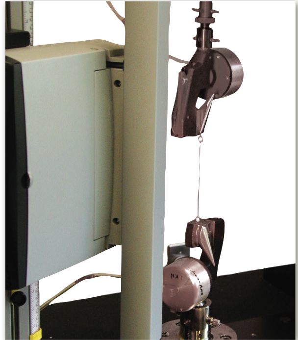
Figure 1: A 5582 frame, 1 kN load cell, 1 kN pneumatic cord and yarn grips and the AVE were used to test Nitinol wire in tension.
