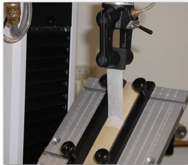
Figure 2: Close up of specimen during peel test using leather as a substrate to simulate the surface properties of skin.
