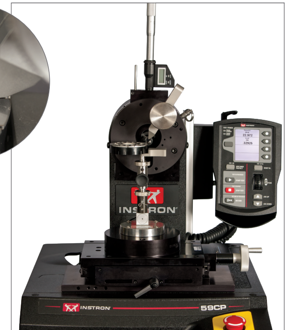
Curved needle test system for testing curved surgical needles to ASTM F3014-14.
