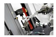
Automated specimen handling systems improve productivity and increase the volume of testing conducted, without additional personnel, by efficiently utilizing valuable instrumentation and modern technology. Increased productivity in the laboratory is a function of intelligent resource allocation. Instron's automated specimen handling systems allow workers to better utilize their time and apply fundamental added value to other projects while maintaining testing throughput.
