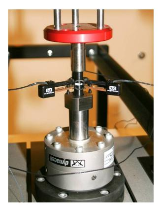
ElectroPuls E3000 testing system used for fundamental research at JKU Linz: Can dynamic loading of a notched, round specimen provide an indication of the service life of a component?
