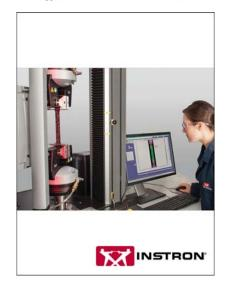
Image and calibration data is supplied by an Instron® Advanced Video Extensometer (AVE). The associated DIC software provides visualization and also saves the data at an adjustable rate of up to 50 Hz in the form of individual images for subsequent analysis in post-processing mode. The software runs independently of other programs, and leverages the graphical layout and tabbed style of Instron's Bluehill® Materials Testing Software – making the user interface familiar and easy to use.
