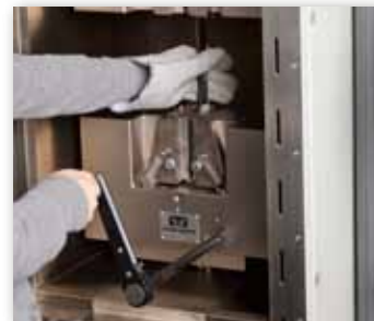
Open Front/Back Allows for Easy Specimen Loading
