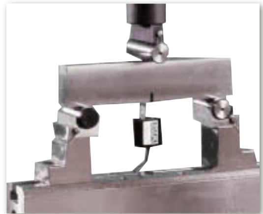
Three-point flexure fixture performing toughness test
