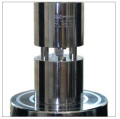
CP105787 Wyoming Modified Celanese Compression Test Fixture
