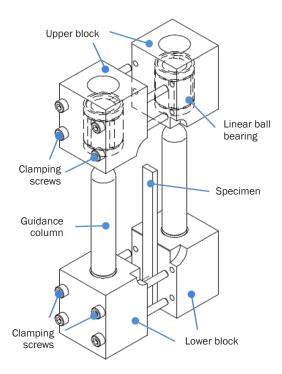
Exploded View of Combined Loading Compression Fixture
