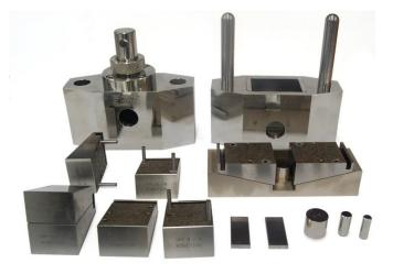
Disassembled IITRI Fixture including Specimen Alignment Fixture and Gage Blocks
