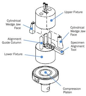
Exploded View of Wyoming Modified Celanese Fixture
