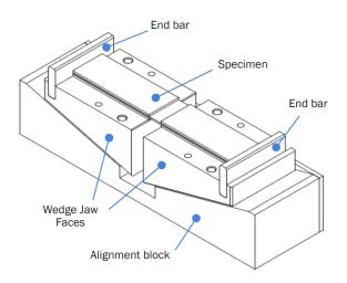
Specimen Alignment Fixture
