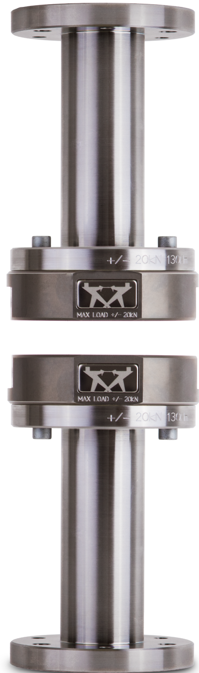
20 kN (4.5 kip) compression platens
