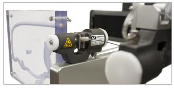
User-supplied tortuous paths and environmental baths can be added to the end of the testing system to simulate friction in a wide variety of physiological environments.
