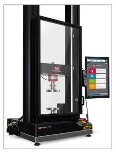
Debris Shield on a Table Mounted System
