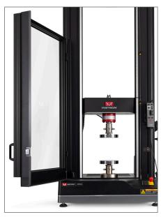
Debris Shield open on a Table Mounted System
