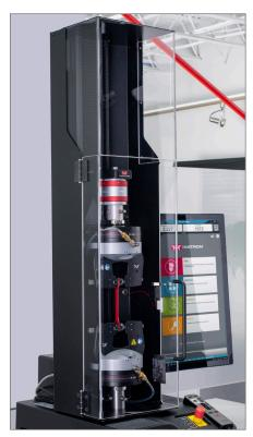
Single Column Shield Fully Encloses Test Space
