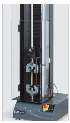
Single Column Shield Fully Encloses Test Space
