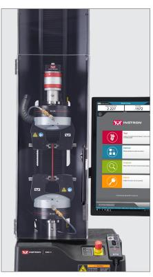
Single Column Shield Fully Encloses Test Space
