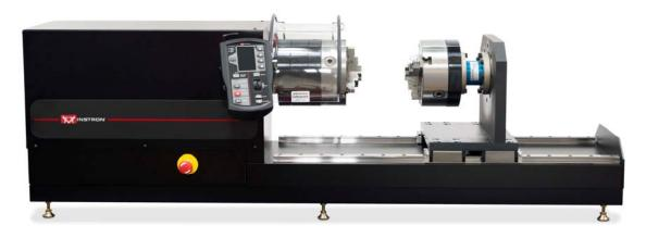
Instron® medium-capacity MT Micro Torsion systems are available in capacities ranging from 565 to 5,650 N-m (5,000 to 50,000 lb-in). The tabletop design requires minimal lab space while offering superior frame stiffness and alignment. Packaged with Instron high-performance control electronics, the MT Series provides highly accurate test data and control for testing fasteners, metal components, and wire rod used in the aerospace, automotive and construction & engineering industries.
