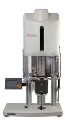
The ability of melted materials to flow under pressure at set temperatures has a fundamental importance in polymer science and technology. The MF50 is especially used by 24/7 laboratories testing several different materials, from fast flowing master batches up to highly viscous rubbery or filled materials, where quick and safe operations have big impact on productivity. It allows multiweight testing procedures.
