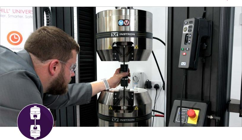
Instron Field Service and Calibration Engineers work directly with ASTM and Nadcap to understand the requirements for materials testing system alignment. We have developed and established alignment services complying with the guidelines and calculations detailed within ASTM E1012 and Nadcap standards.
