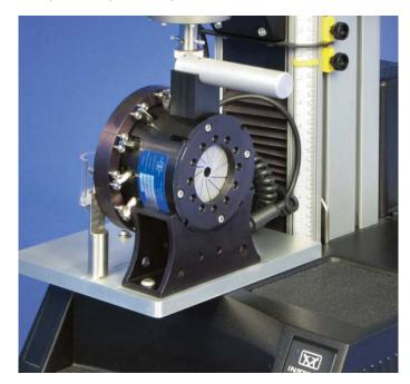
Using a specialist fixture incorporating a segmental compression mechanism, it is possible to determine radial stiffness, chronic outward forces during expansion and compression, as well as the radial reactive force during compression of different devices. This approach provides uniform application of radial forces for easy comparison
