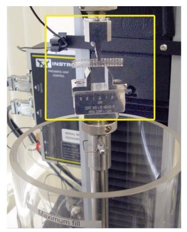
Techniques for gripping have often revolved around using jaws with adjustable clamping forces, such as pneumatic or hydraulic grips, or specialist strain measurement is carried out using a non-contacting video based extensometer.
