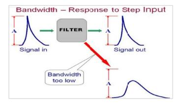
"It is difficult to give an exact number for the minimum required bandwidth of a quasi-static testing machine, but it is important to ensure that the response being observed during a test is not limited by the bandwidth of the testing machine. On the other hand, an excessively high bandwidth can be detrimental to the system's performance as accuracy may degrade and noise may increase."
