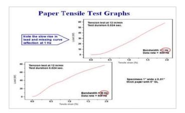
Peel Tests – Comparison of 1 Hz vs. 10 Hz Bandwidths
