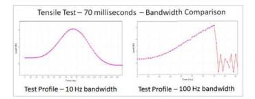
The Instron 6800 Series testing systems offer 10, 100, and 500 Hz bandwidth settings and the higher bandwidths should be used for test events less than 40 msec or tests lasting less than 2 seconds.
