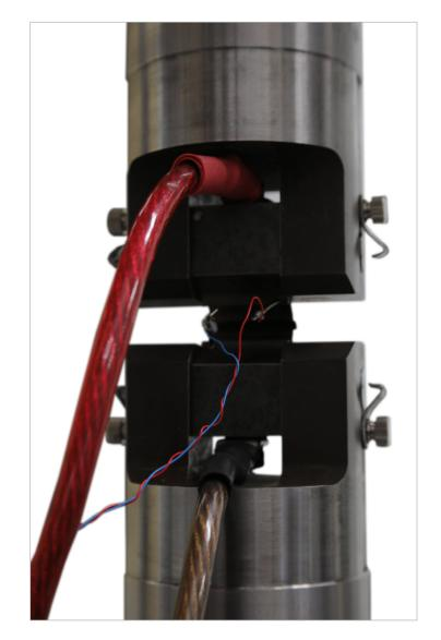
Test control and method set up are similar to mechanical compliance-based methods and raw data is stored in the same way. Signal noise depends greatly on the preamplification and conditioning of the DCPD system, so an additional averaging feature is available to stabilize readings during crack growth.
