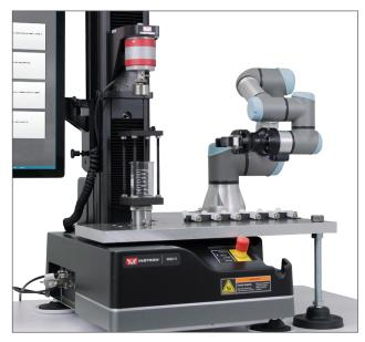
The CT6 is compatible with Instron's 6800 and 5900 systems. It mounts easily to a new system or can be retrofitted onto an existing system in the field.
